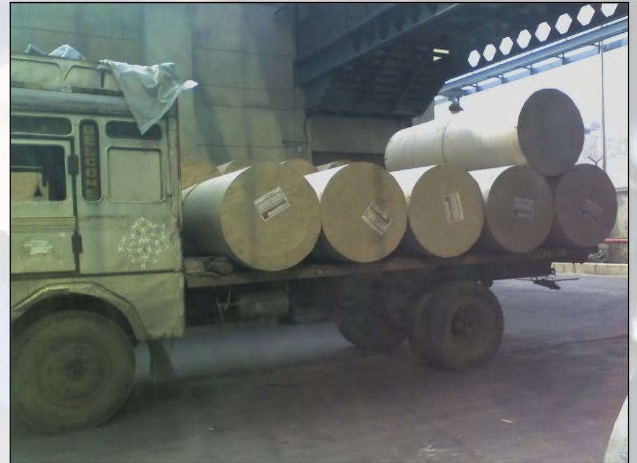
Single layer loading (12 reels)
